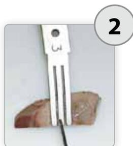
Cut other side of the central fork to obtain a pre-set thickness specimen.
