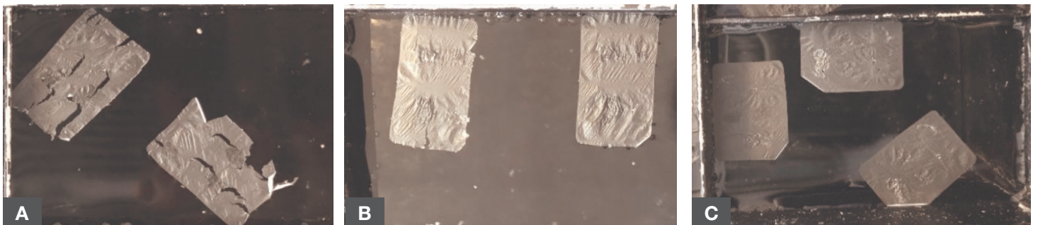
Figure 2. (A) Thin section of a pork belly specimen prepared with a conventional tissue processor (without defatting pre-treatment). (B) Thin section of a pork belly specimen prepared with a conventional tissue processor (with defatting pre-treatment). (C) Thin section of a pork belly specimen prepared with Revos (without defatting pre-treatment). Specimens prepared using Revos showed fewer cracks even without defatting pre-treatment.
